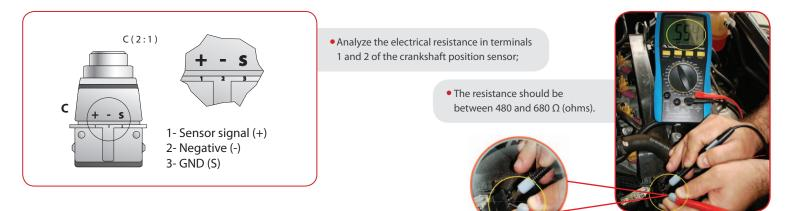
Note: Each injection system is provided with a crankshaft position sensor with a specific resistance value, which varies pursuant to the gauge and the number of turns of the coil.
