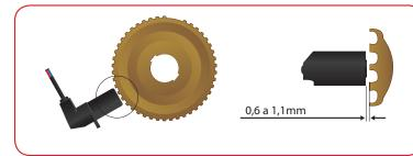
Only a minority of vehicles is provided with devices to adjust the position against a majority of them, in which they are fixed and do not allow this adjustment. Therefore, if the sensor does not meet the recommended value, the operator should verify if the mounting bracket is not damaged.
